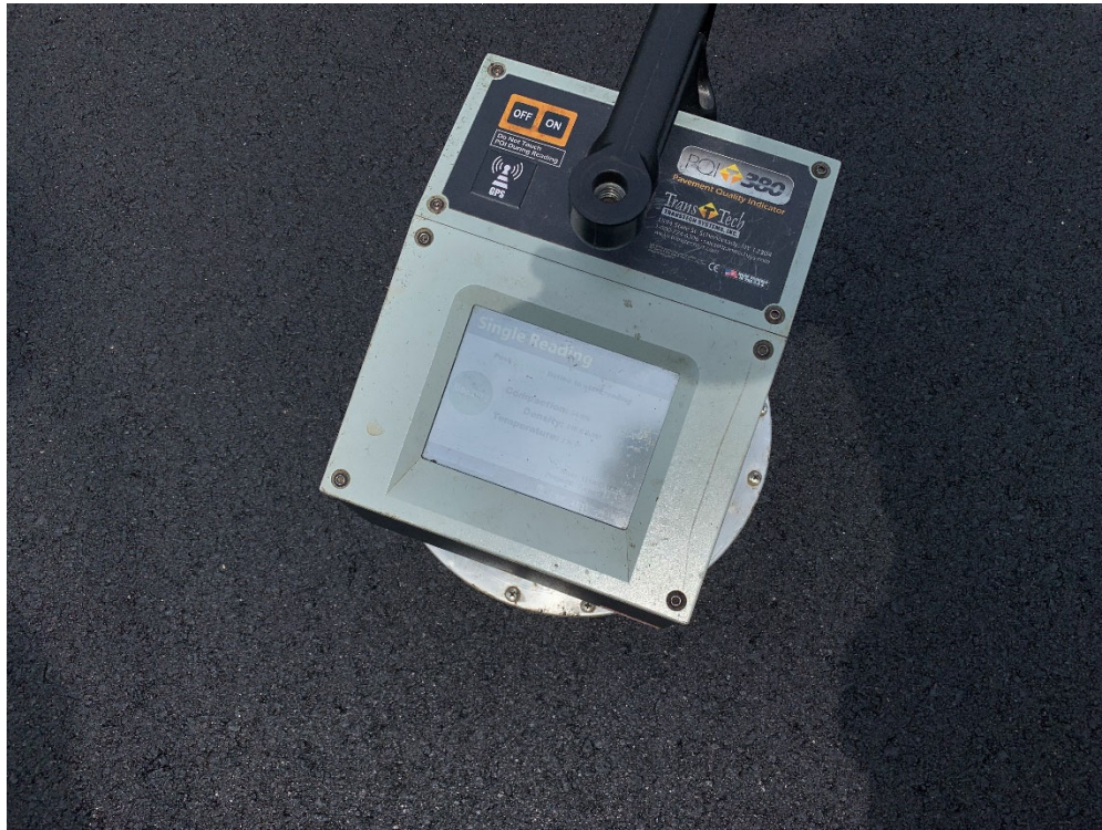
Photo 7 – Compaction of 94.9% and density of 148.9 pcf on surface pavement in northwest lane near 198 Tuttle Road.
