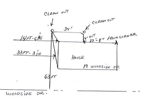
Town, City of: Cumberland Date Installed 5-20-83 Street Woodside Drive Type, Size of Service Pipe 6 Q.V.C. Dwelling No. #21 Connection at Sewer Main Tee Occupant Depth, End of Service Pipe Owner MARK R. EATON Length of Service Pipe Laid 13' C-5-C935 Measured, Located By Q.C.Q.T. A.J. Bronding Sons Project Contractor LOCATION DIAGRAM House #21 99' Remarks:
