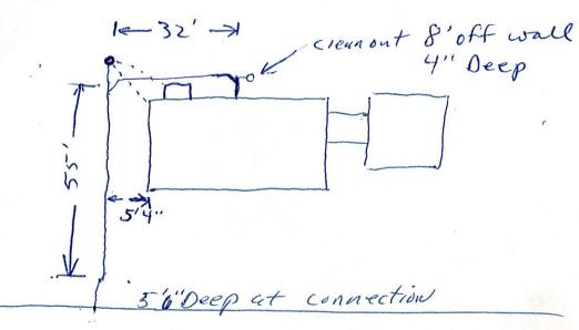
SANITARY SEWER SERVICE LUCATION Town, City of: Cumberland Street Meadowniew Goad ate Installed 8-16-83 Dwelling No. Type, Size of Service Pipe 6" PY.C. Occupant Connection at Sewer Main TEE Owner Depth, End of Service Pipe Length of Service Pipe Laid 21' Measured, Located By QBc GT J.J. Gronding o' Sons Project Contractor LOCATION DIAGRAM House #X6 Remarks:
