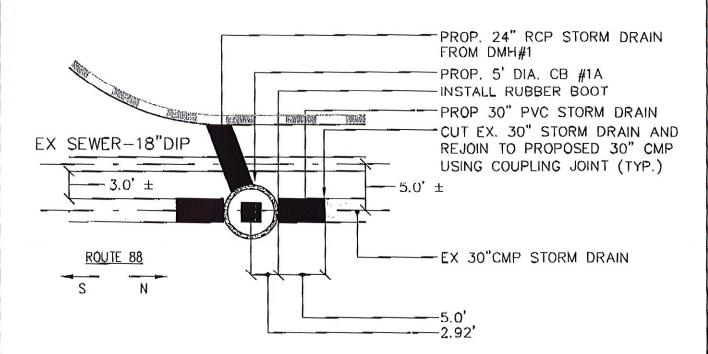
NOTE: TEST PITS NEED TO BE DONE PRIOR TO ORDERING STRUCTURE TO VERIFY SEPARATION BETWEEN SEWER MAIN AND STORM DRAIN IS 5 FEET. IF SEPARATION IS LESS THAN WHAT IS SHOWN CONTRACTOR TO PROVIDE FIELD SKETCH TO ENGINEER FOR REVIEW OF STRUCTURE & PIPE ALIGNMENTS.
