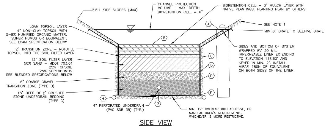
1. THE SIDESLOPES SHALL BE STABILIZED WITH A MIN. OF 4" LOAM, EROSION CONTROL BLANKETS SC150BN BY NORTH AMERICAN GREEN OR APPROVED EQUAL AND A CONSERVATION SEED MIX.
