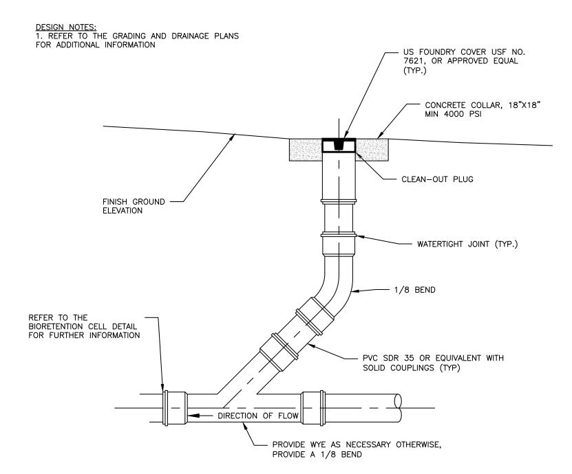
CLEANOUT DETAIL WITH CONCRETE COLLAR NOT TO SCALE
