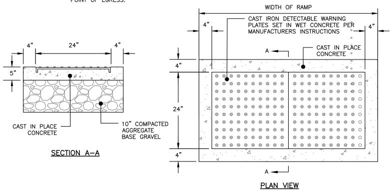
SIDEWALK RAMP DETECTABLE WARNING PANEL NOT TO SCALE
