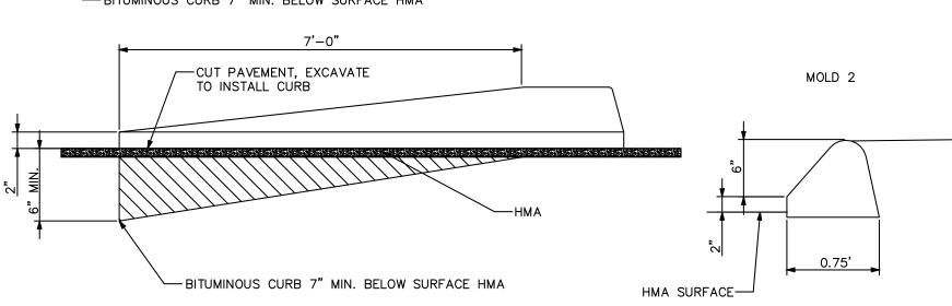
SLIPFORM BITUMINOUS CURB DETAIL
