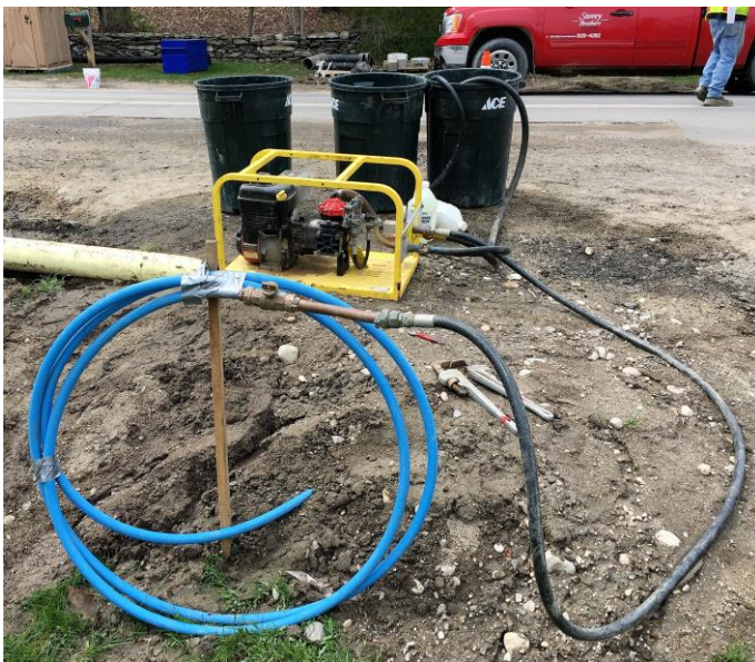
Pump used for hydrostatic pressure test through the chlorination tap installed at in front of 161 Middle Road.
