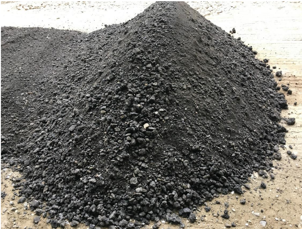
Close-up of screened pavement millings placed over Type D subbase gravel in lieu of Type A crushed gravel.
