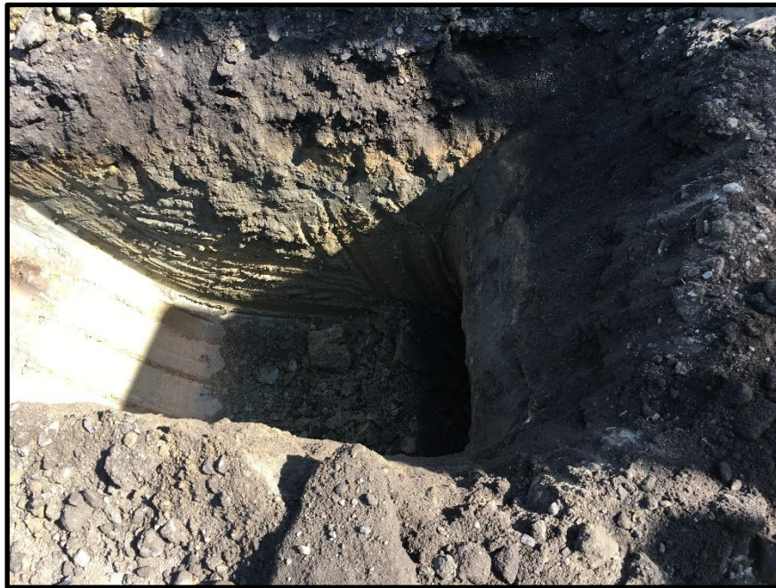
Photograph 4 - Friday, September 15 th – Test Pit 9 at STA 47+50 10' Left – Did not reach ledge at a depth of 45 inches below the milled pavement. Gravel/clay interface was about 18 inches below top of the 2 inches of milled pavement remaining. This area was in a “partial” box cut area.
