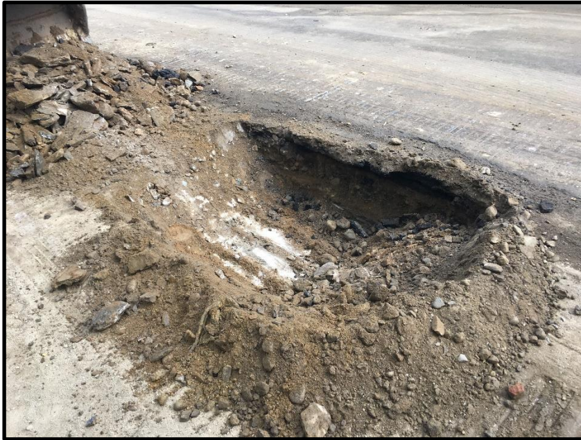
Photograph 3 – Friday, September 15 th - Test Pit 3C at STA 35+30, 10' Left - Encountered ledge 18-inches below the top of the milled pavement. About 4 inches of pavement had been milled off leaving about 3 inches. This area is in a “full” box cut area.
