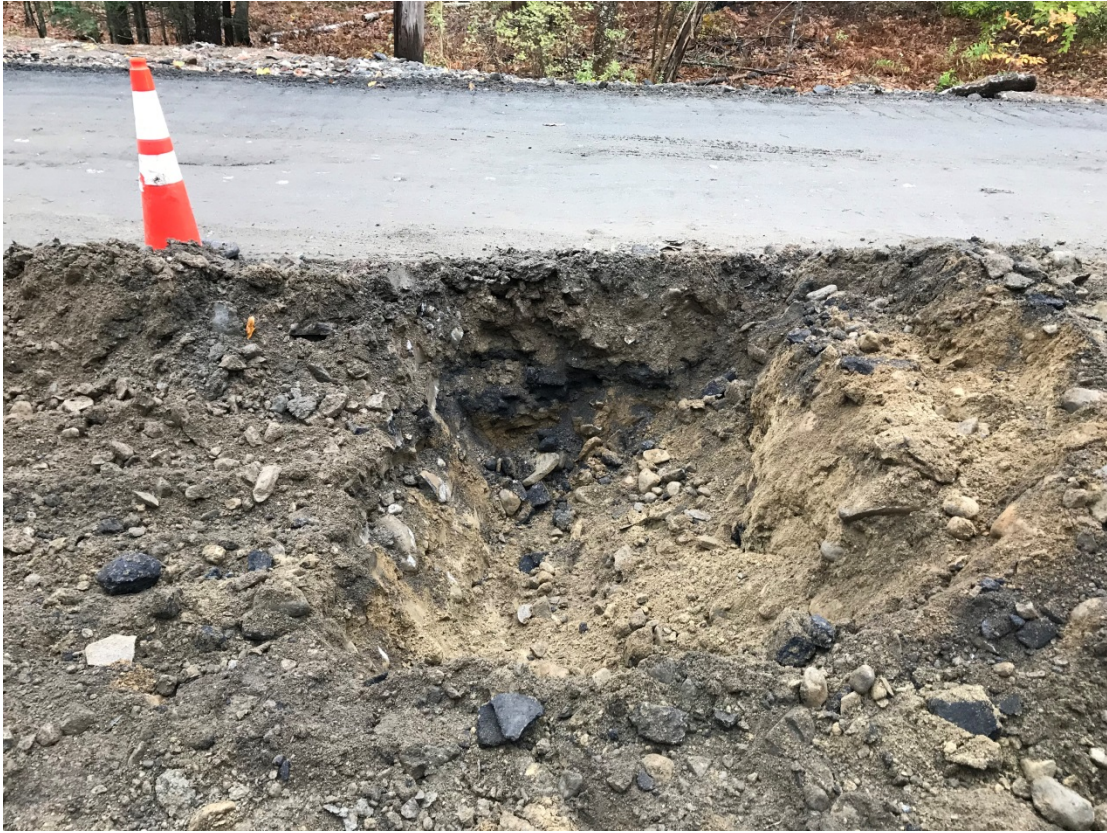
Photo 3 – Test pit 2 to determine existing depths of pavement and gravel. Samples of existing gravel were collected.
