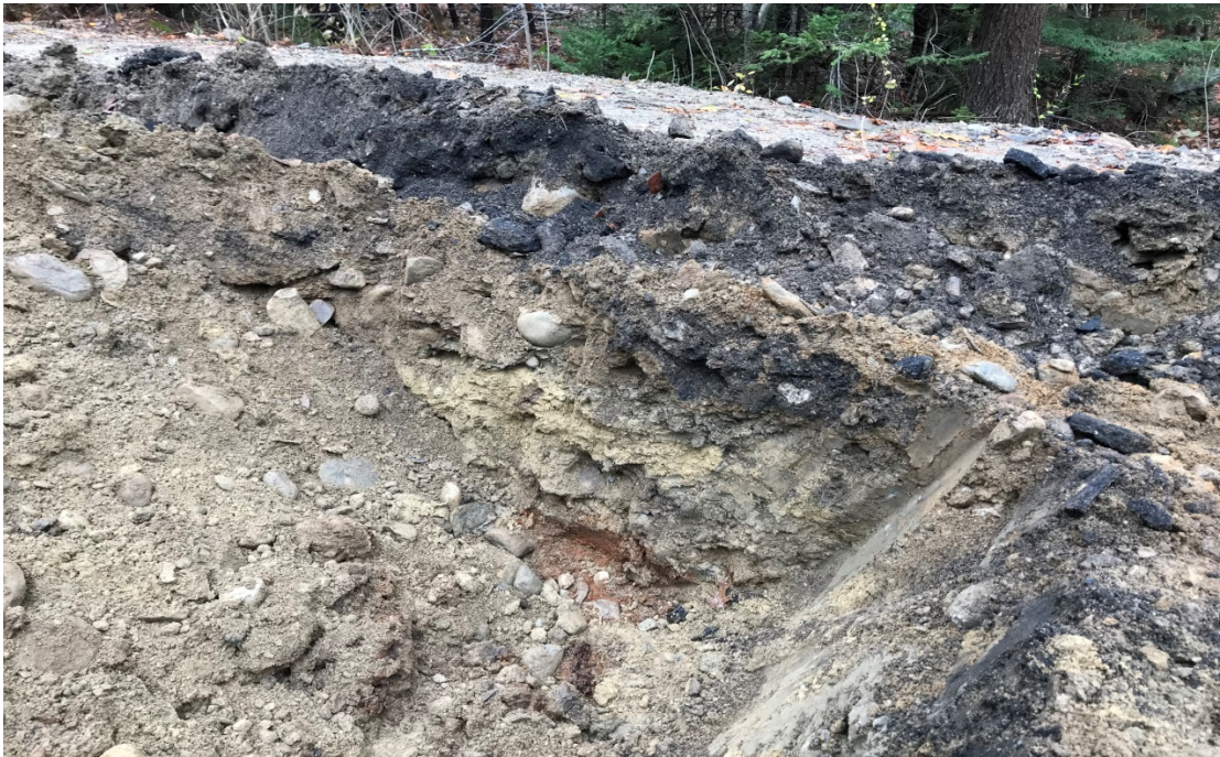
Photo 4 – Test pit 3 to determine existing depths of pavement and gravel. Samples of existing gravel were collected.
