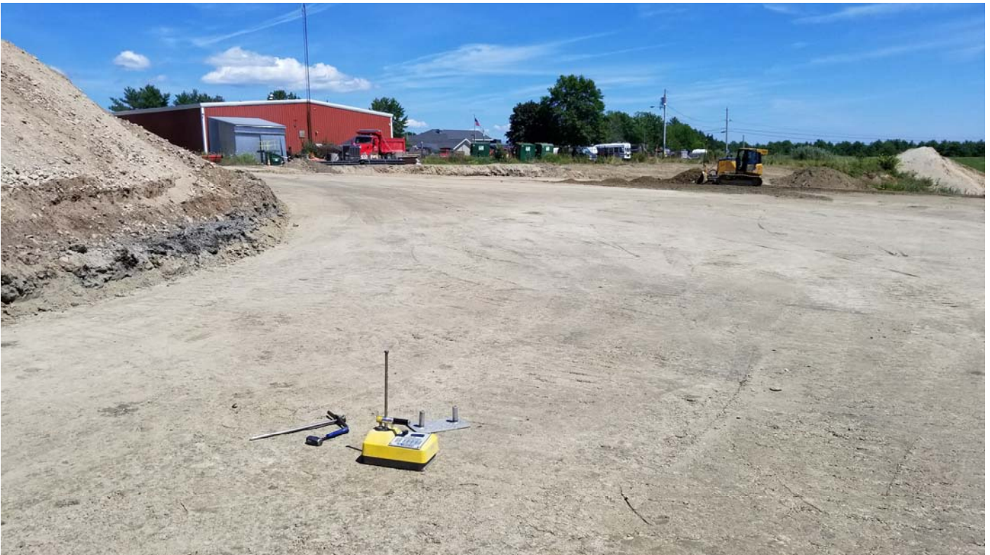
Density testing for the twelve-inch lift was completed near the end of day Friday.
