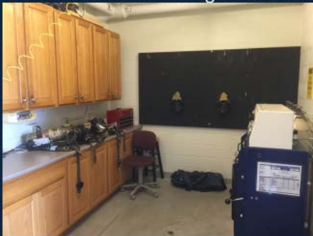
Separate room for Breathing Air and Compressor System to fill the tanks. Work shop to repair breathing apparatus.
