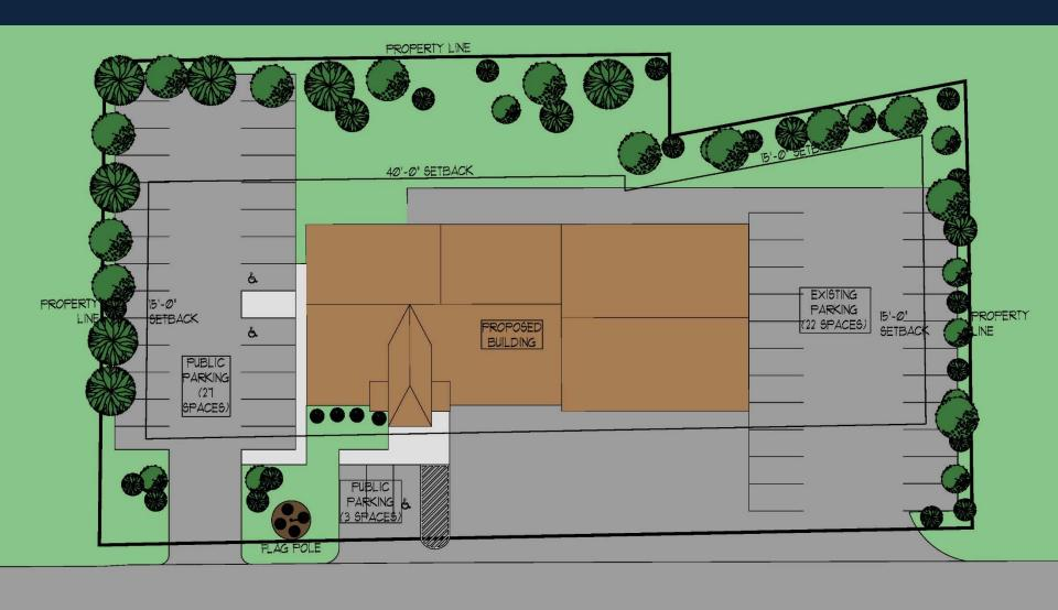
Proposed Site Plan with 30 new Public Parking Spaces, Site Buffering, and Drainage
